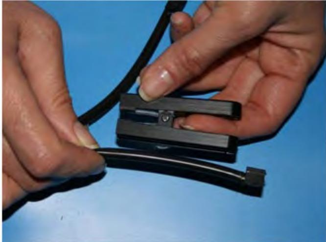
Push the fiber into the large groove along the length of the clip making sure the collar is in close proximity to the end of the clip.
