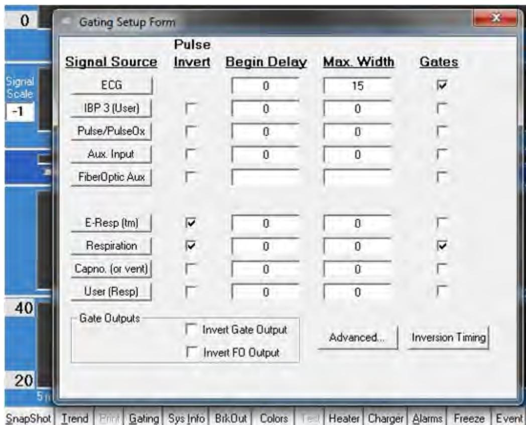
Click the Gating key to open the GATING SETUP window. This window provides a means to include one or more signals in the gating algorithm. In the window above, both ECG and respiration gates must be satisfied for generation of an output gate (white dot).
