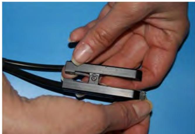
To remove the fiber, grasp the fiber with the thumb and index finger as shown. Push the fiber to move the collar away from the clip. Then grasp the collar with the thumb and index finger and remove the collar from the clip.
