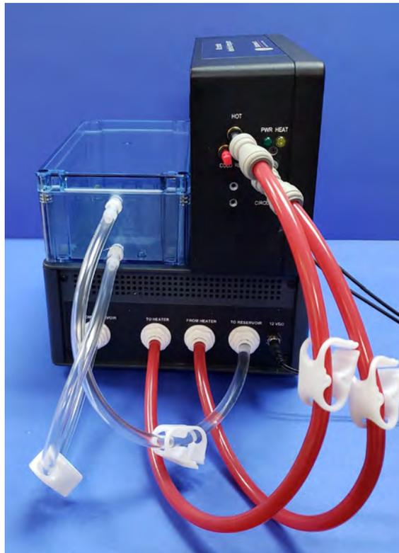
Water is circulated through the closed loop system at constant flow (1.5 GPH) and low pressure (5 psi). PC software controls the temperature of the water being circulated through a heating pad or blanket covering the animal in the magnet bore. Control is based on a user defined set point for the water output temperature, the heating pad temperature or the animal temperature.
