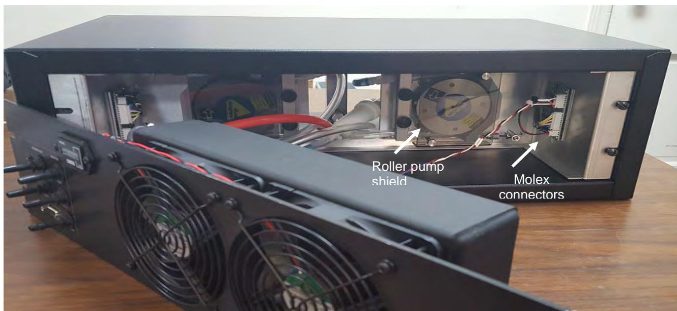
When removing tubes from the Heater Module, clamps can be useful on the 3/8" OD tubing. Plugs can also be used on the Heater Module ports.
