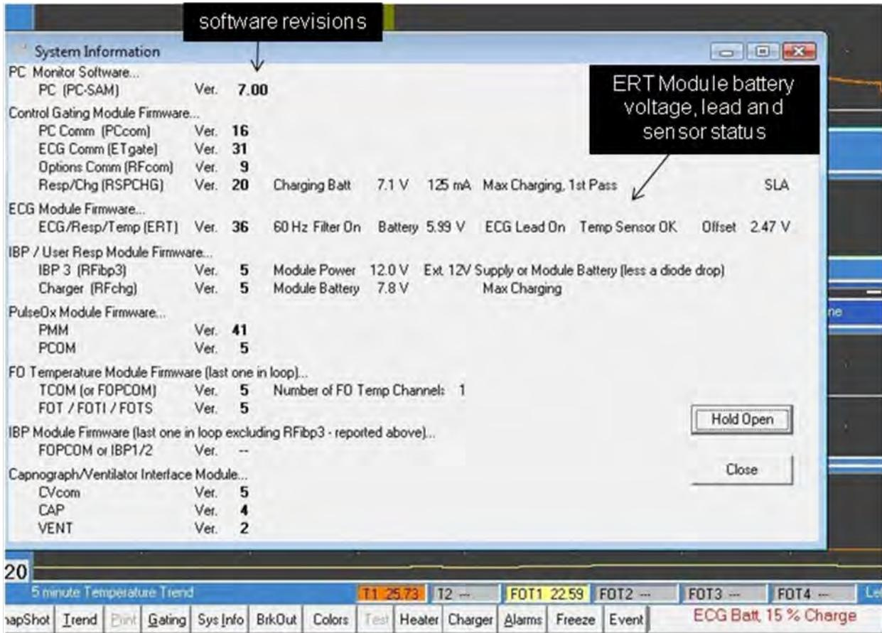
ERT Module status includes the 50Hz/60Hz notch filter setting, battery voltage, ECG and temperature lead status and offset voltage.
