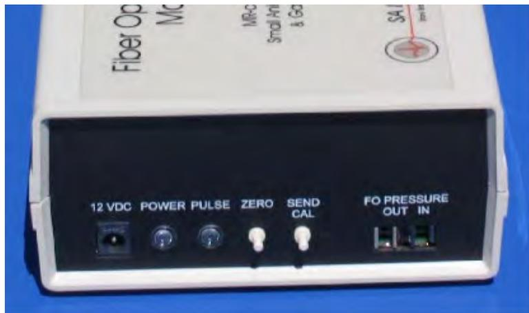
If the yellow light is on continuous and a pressure sensor is connected, press the “send Cal” button to store the new gage factors in EEPROM memory. The yellow light should then begin flashing to indicate a zero is necessary.
