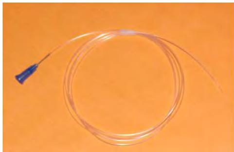
tubing. Cannulas can be constructed in a number of ways using needles, tubing and Luer connectors.
