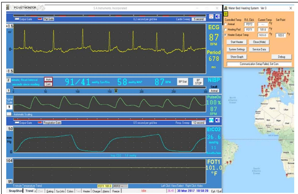
The message area at the bottom of the window gives system status and error messages. On the left of the window the user can select the method of control, the temperature probe in use for measuring the animal or heating pad and the temperature set point. Click in the box to change between available probes. Note the control selection is grayed out or made inactive if the probe selected does not have a valid temperature reading. Measured values for fluid output and temperature probes are displayed.
