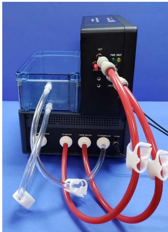
Water is circulated through the closed loop system at constant flow (1.5 GPH) and low pressure (5 psi). The Heater Module's internal microprocessor controls the temperature of the water being circulated through a heating pad or blanket covering the animal in the magnet bore. Control is based on a user defined set point for the water output temperature, the heating pad temperature or the animal temperature.
