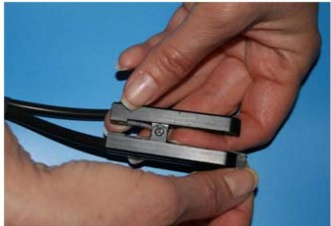
To remove the fiber, grasp the fiber with the thumb and index finger as shown. Push the fiber to move the collar away from the clip. Then grasp the collar with the thumb and index finger and remove the collar from the clip.
