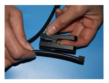
Grasp the collar with the thumb and index finger and insert the collar groves into the tracks of the clip. Use the index finger to push the collar to the end of the clip opening.
