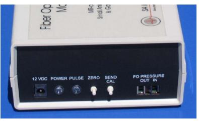
If the yellow light is on continuous and a pressure sensor is connected, press the "send Cal" button to store the new gage factors in EEPROM memory. The yellow light should then begin flashing to indicate a zero is necessary.
